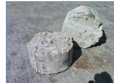
c) Cored Samples with Recycled In-Situ Materials
